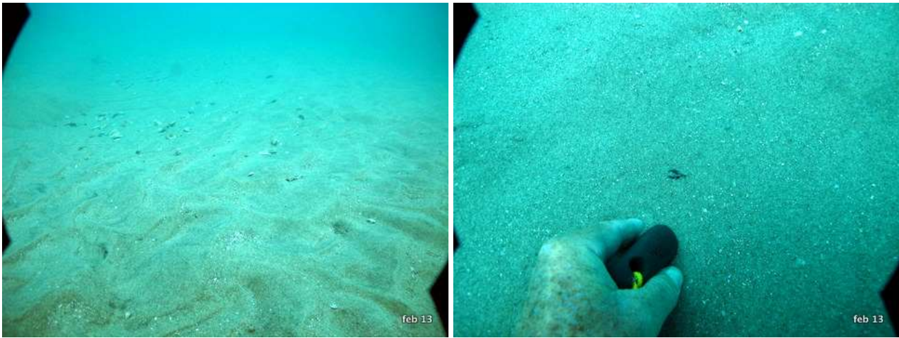
Figure 6 Photo point C: (left) showing large and small wave ridges, (right) showing excavation hole filling in completely with loose sand as trowel is thrust in full length. Depth -10.1m
