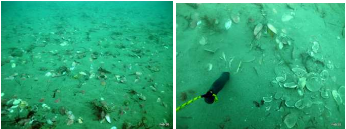
Figure 24 Photo point N: (left) showing significant shell content, (right) showing excavation hole filling in with loose sand as trowel is thrust in full length and shell excavated to left from hole. Depth -12.6m.
