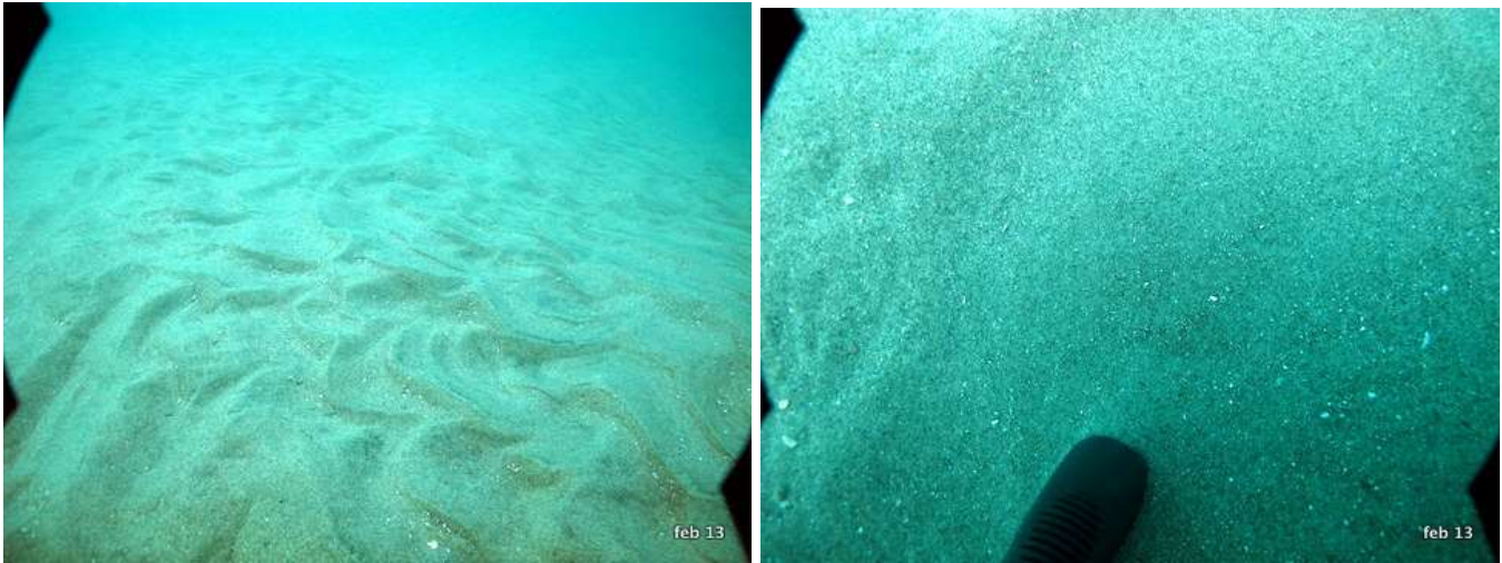
Figure 7 Photo point D: (left) showing sand wave ridges, (right) showing excavation hole filling in with loose sand as trowel is thrust in full length. Depth -8.1m.
