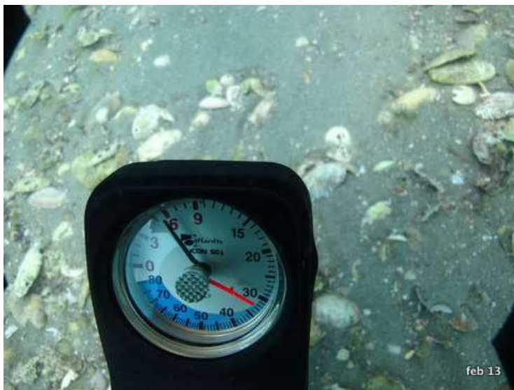
Figure 9 Photo point F: showing high shell content and armouring of seabed. Depth = -2.8m. Note depth gauge is an uncorrected high tide reading.
