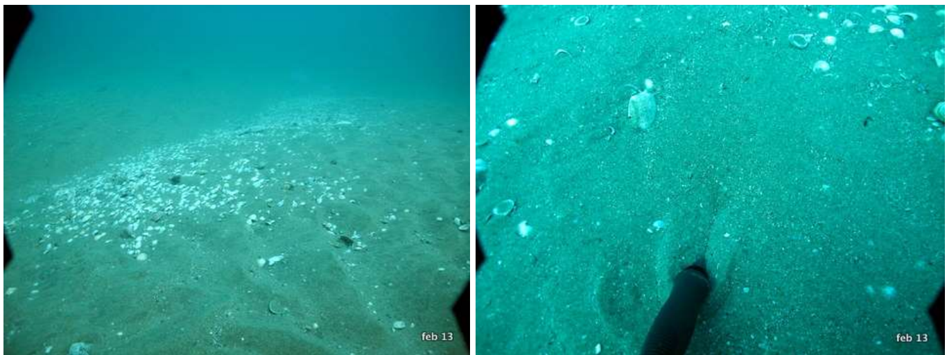
Figure 5 Photo point B: (left) showing sand wave ridge, (right) showing excavation hole filling in with loose sand as trowel is thrust in full length. Depth -11.9m.
