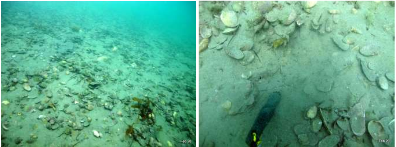
Figure 26 Photo point P: (left) showing significant shell content, (right) showing excavation hole filling in with loose sand as trowel is thrust in full length and shell to left excavated from hole. Depth -8.4m.
