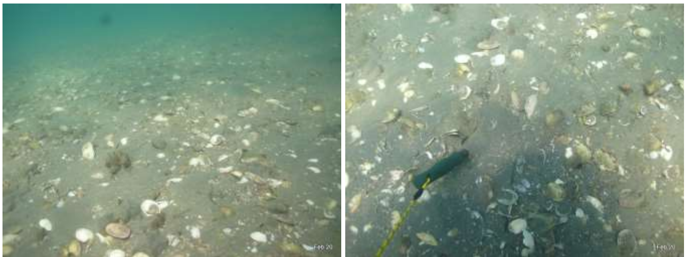
Figure 21 Photo point Z: (left) showing high shell content with some mobile sand, (right) showing excavation hole filling in with loose sand as trowel is thrust in full length and high shell content.. Depth - 3.4m.
