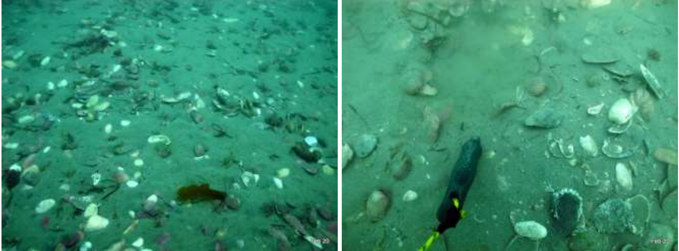
Figure 25 Photo point O: (left) showing significant shell content, (right) showing excavation hole filling in with loose sand as trowel is thrust in full length and shell to left excavated from hole. Depth -10.4m.
