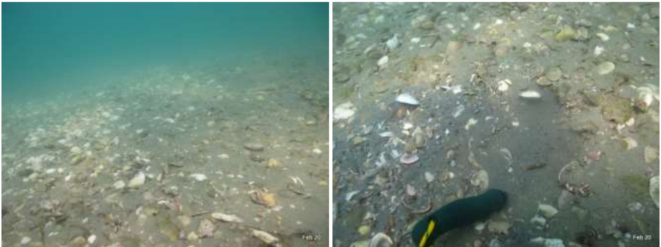
Figure 20 Photo point Y: (left) showing high shell content, (right) showing excavation hole filling in with loose sand as trowel is thrust in full length and high shell content. Depth -3.5m
