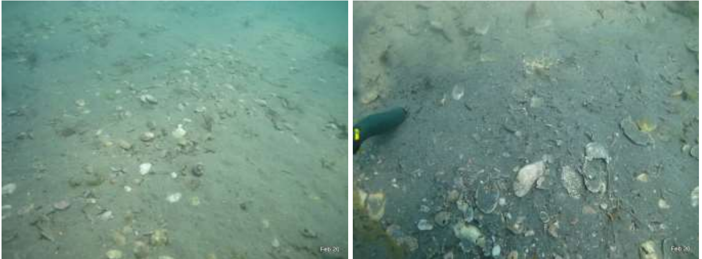
Figure 17 Photo point V: (left) showing significant shell content, (right) showing excavation hole filling in with loose sand as trowel is thrust in full length and shell fragments to the left excavated from the whole. Depth -4.9m.
