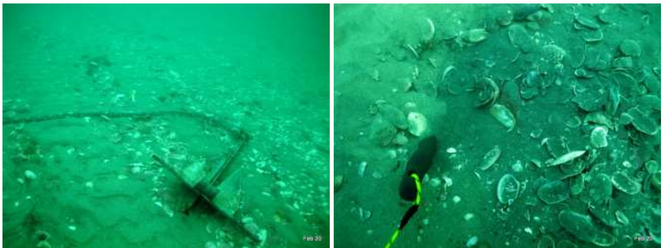
Figure 22 Photo point L: (left) showing significant shell content, (right) showing excavation hole filling in with loose sand as trowel is thrust in full length and shell to left excavated from hole. Depth -15.6m.
