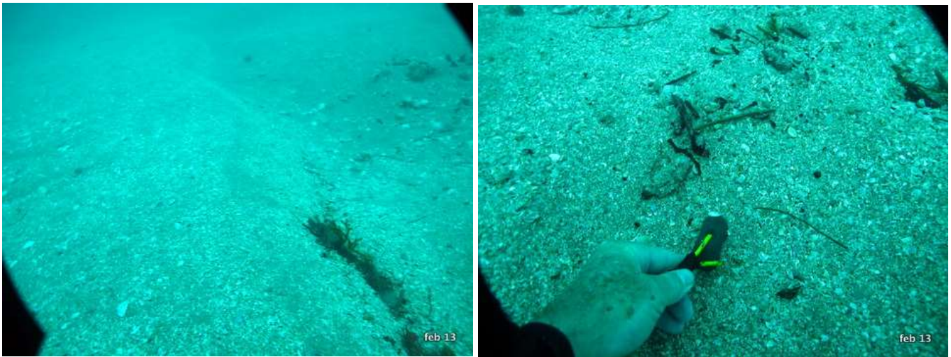
Figure 14 Photo point K: (left) showing sand wave ridge, (right) showing excavation hole filling in with loose sand as trowel is thrust in full length. Depth -13.2m.
