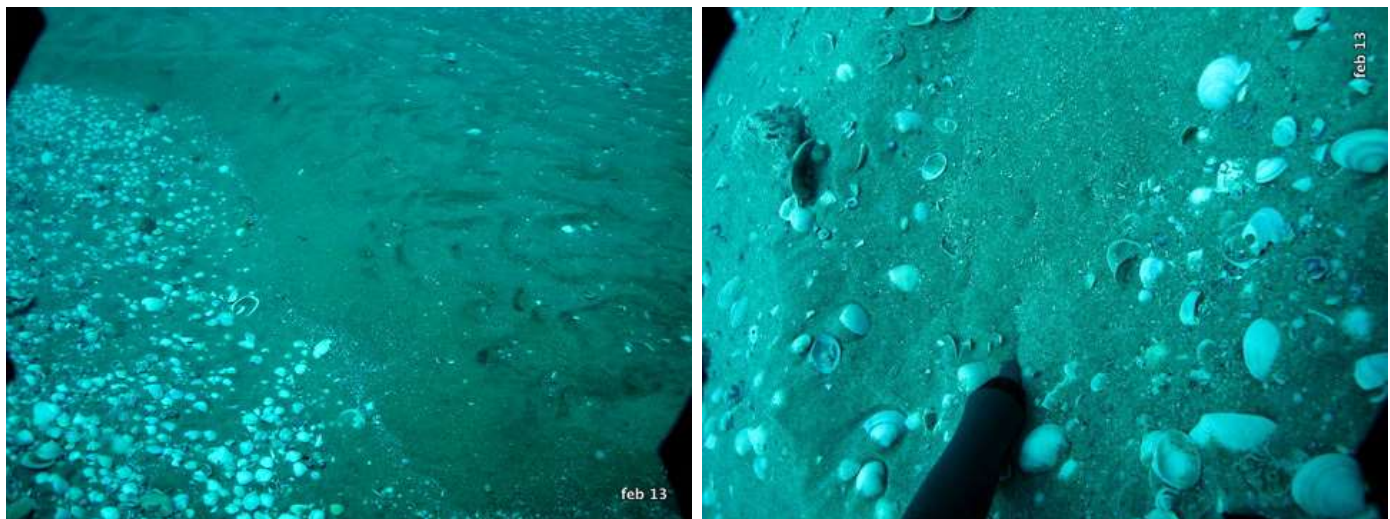
Figure 4 Photo point A: (left) showing sand wave ridge, (right) showing excavation hole filling in with loose sand as trowel is thrust in full length. Depth -14.1m.
