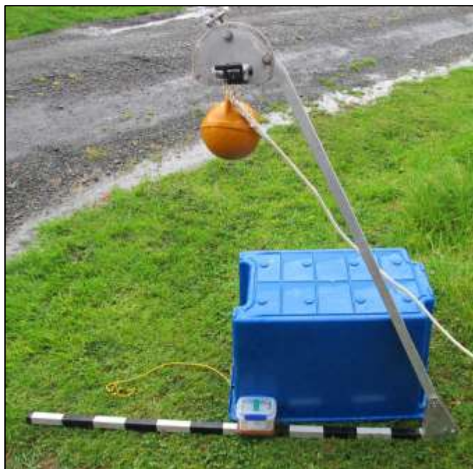
Figure 2 The baited underwater video (BUV) apparatus with GoPro camera mounted at the top of the frame facing down
