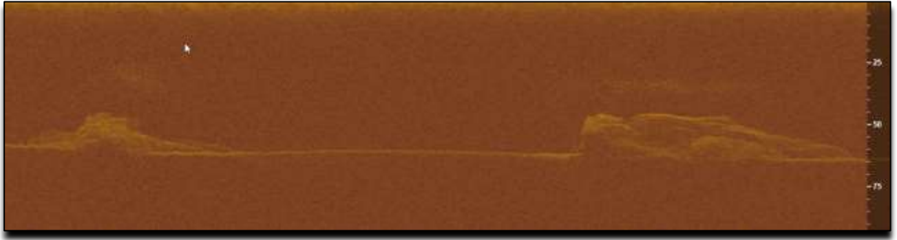
Figure 22 A sonar profile view of the two reefs that make up the outer reef (note the depth scale on the right hand side and a faint view of fish schools hovering over the top of the reefs).
